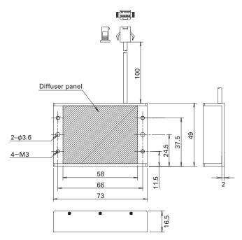
Fig. 5: External diagram of the flat-type LED light
