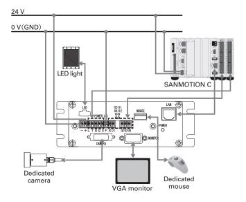
Fig. 7: Example of system connection for the "VS-AS"
