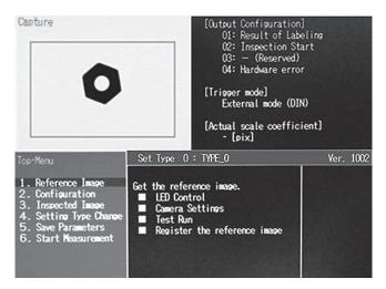
Fig. 8: Example of the setting menu screen
