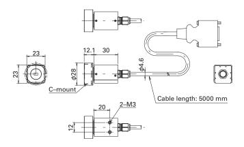
Fig. 3: External diagram of the camera
