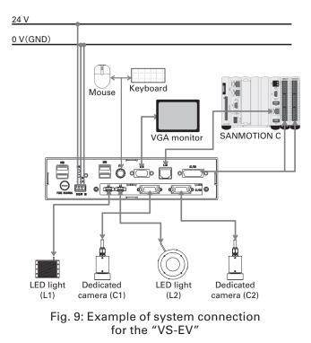
This unit comes preinstalled with "EV-Plus"- dedicated image processing software for VS-EV. This software makes it possible to flexibly support various inspection applications.
